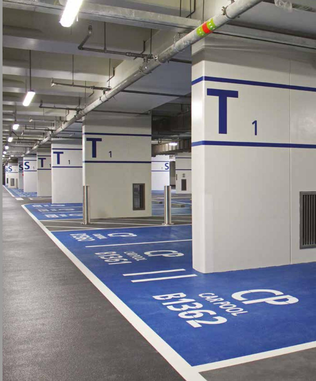
A high volume of vehicles traversing a car parking structure over time can lead to dynamic loading, where vibrations impart through the decks into the structure, increasing the risk of movement across all construction, expansion and movement joints within the frame of the structure and decks themselves.
