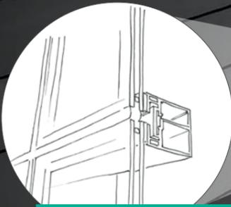
Tremco and illbruck commercial glazing sealants, gaskets and tapes integrate with air barriers and transition assemblies at the window-to-wall interface, creating an air- and water-tight wall proven in extreme weather conditions.
